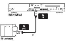
1 Use a DV cable (not supplied) to connect the DV jack of your DV camcorder/video deck to the front panel DV IN jack of this recorder.
